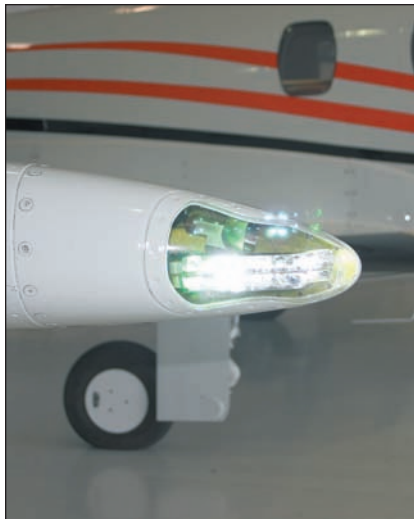
LED position and strobe lights at the wingtips have 10,000-plus-hour service lives. This is part of Eclipse's drive to improve dispatch reliability by several orders of magnitude over current production light jets.
