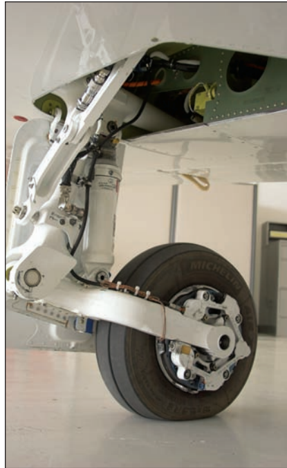
Generous ground effect and long-travel, trailing-link main landing gear all but eliminate any possibility of making a bad landing. The landing gear are electrically actuated. The only hydraulic system on the aircraft is the wheel brakes.
