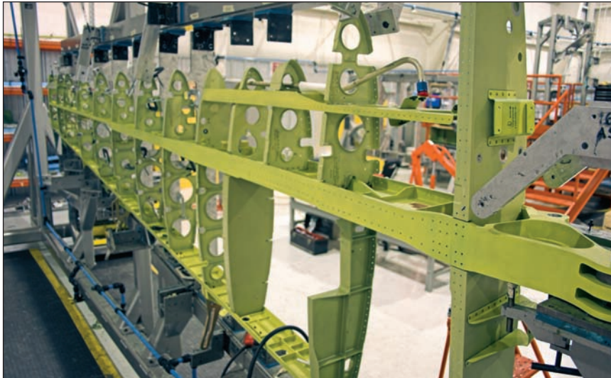
Production aircraft wings will be built by Fuji Heavy Industries. The interior structure has very few parts outside of the one-piece main- and aft-wing spars and a dozen or so one-piece chord-wise ribs all produced by high-speed CNC mills.
