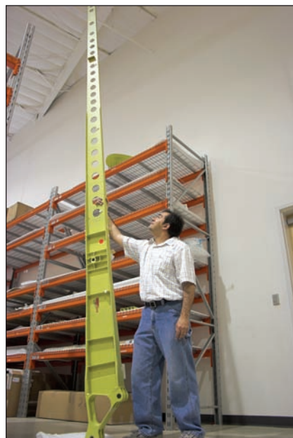
The one-piece main spars are unusually stout for a 5,650-pound MTOW aircraft. The Eclipse 500 should sail through static and fatigue tests at South West Research Institute in San Antonio.
